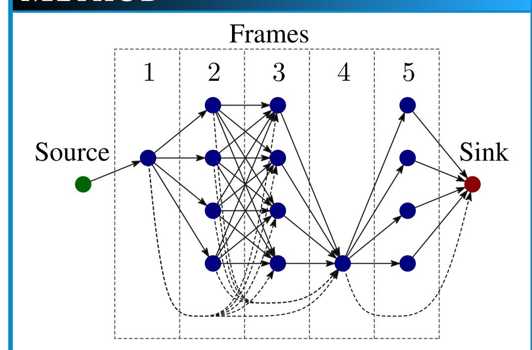
The cost is interpreted as a directed acyclic graph with weights on the nodes and edges. The nodes encode candidate positions, and the edges the transition costs between candidates. Additional edges (dashed) allow occlusion transitions which skip frames.
