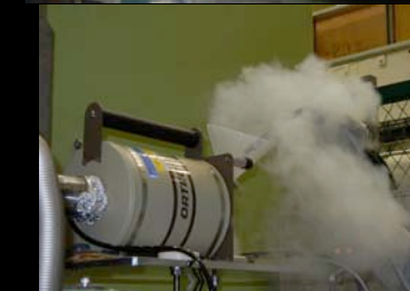
Ortec, POPTOP type, GMX φ=50mm, length=50mm
